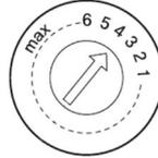
Take off the lid of the rinse aid dispenser and adjust the dial to the desired level. The factory setting is "4".
