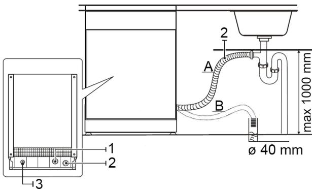
1 Water inlet    2 Drain pipe    3 Mains cable
