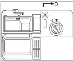
If the warning LED does not light up, you can estimate the amount of remaining rinse aid to the optical level indicator (D) next to the dispenser.
