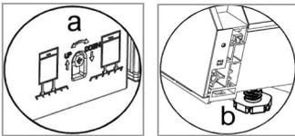
The maximum adjustment height of the feet is 50 mm.
