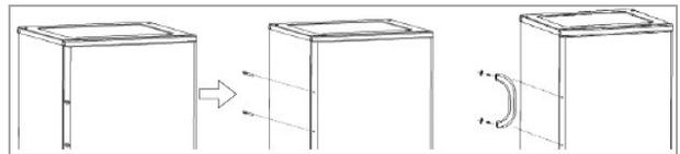
Attach the door handle by removing the cover caps from the door outer side and tighten the handle with the delivered screws into the underlying holes. Put the included screw covers on.
